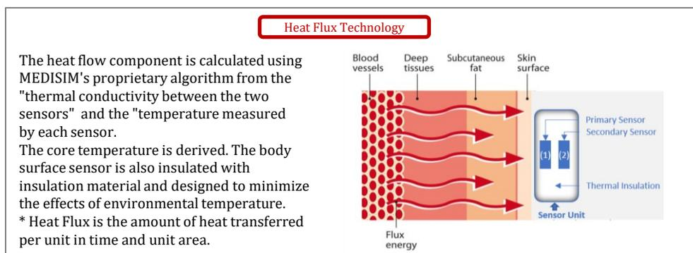
Figure 1: Measurement Method
